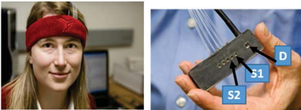
Figure 4-6. On the ISS device, the light sources and detectors embedded into two rubber probes. A detector and set of light sources (s1, s2, s3, and s4) are placed on the head.
